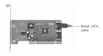
Figure 3. Connecting the Serial ATA cable
